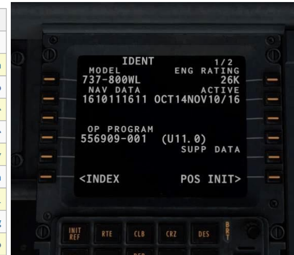
Modern FMS installed on a 737-800WL
