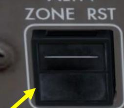
Zone Temperature Controller Reset Switch & SYSTEM FAULT Light
