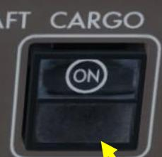
Aft Cargo Heat Switch & TEMP Light
