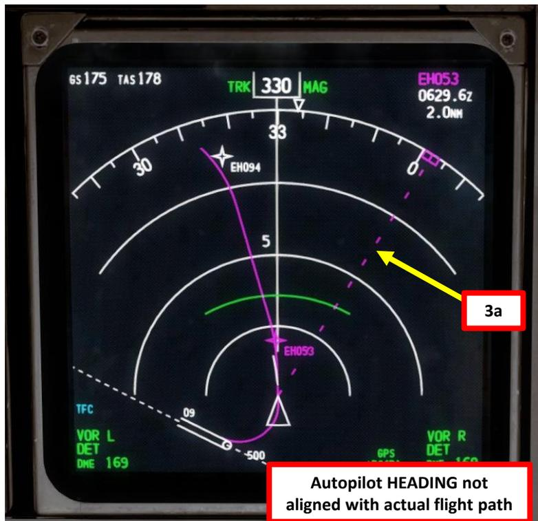
Autopilot HEADING not aligned with actual flight path
