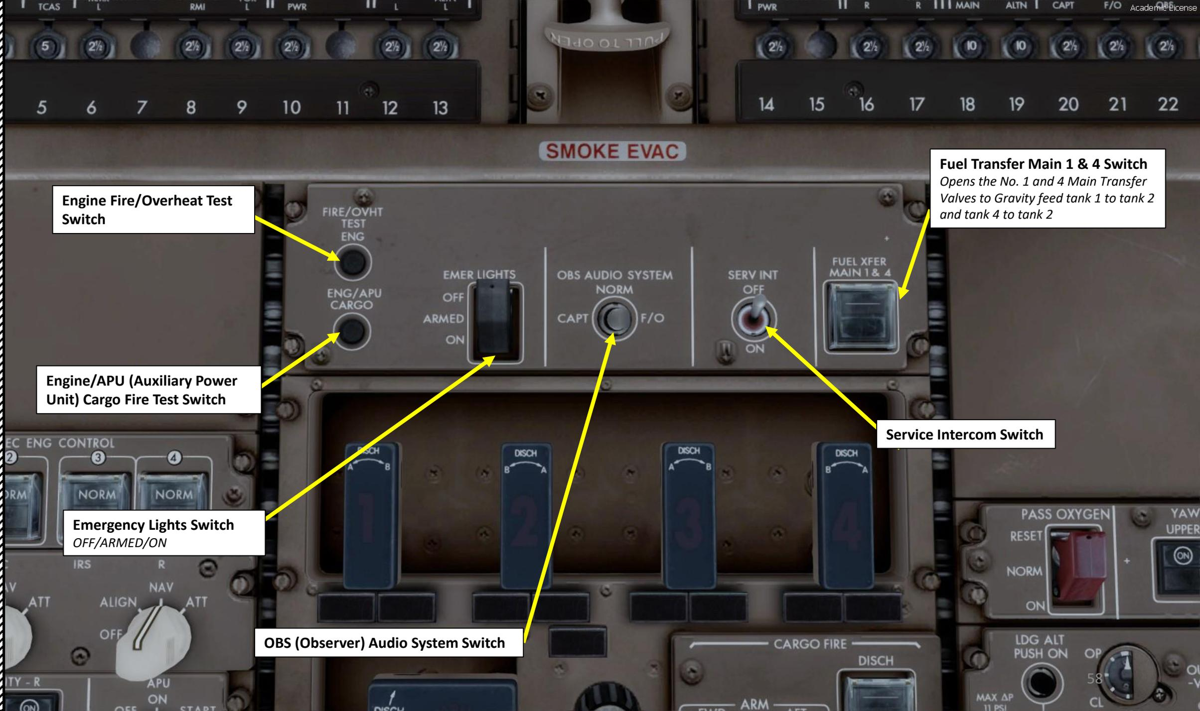
Engine Fire/Overheat Test Switch
