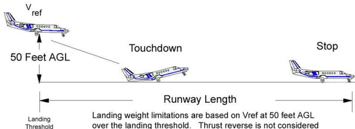
Landing weight limitations are based on Vref at 50 feet AGL over the landing threshold. Thrust reverse is not considered when determining maximum landing weight based on runway limitations.
