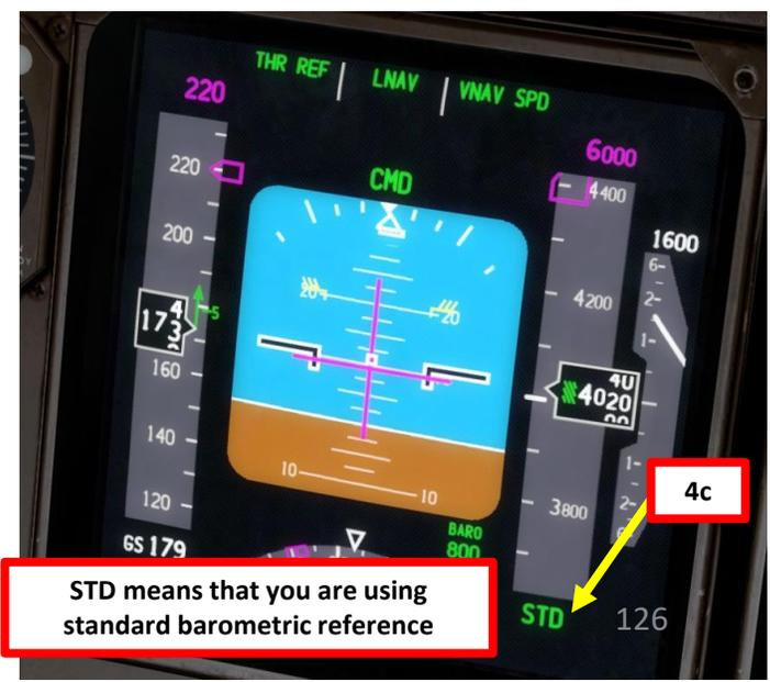
STD means that you are using standard barometric reference
