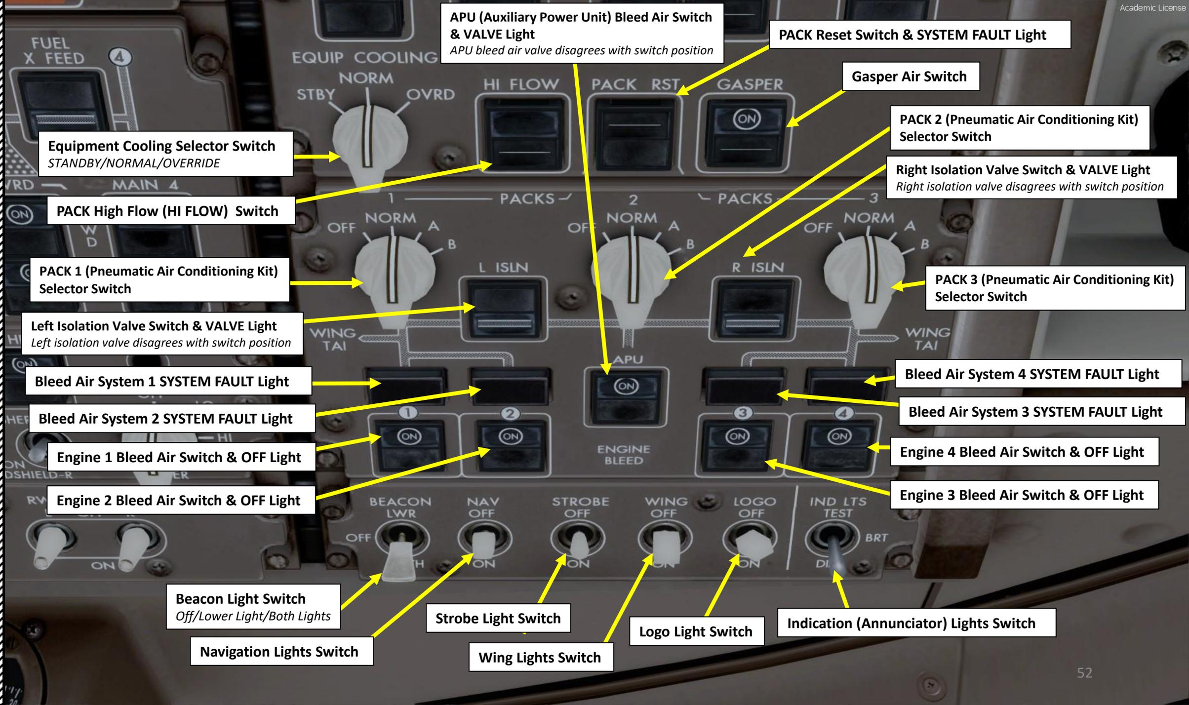
**APU (Auxiliary Power Unit) Bleed Air Switch & VALVE Light**
