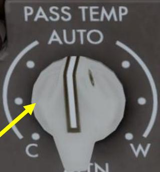
Flight Deck Temperature Control (Cold/Auto/Warm/Alternate)
