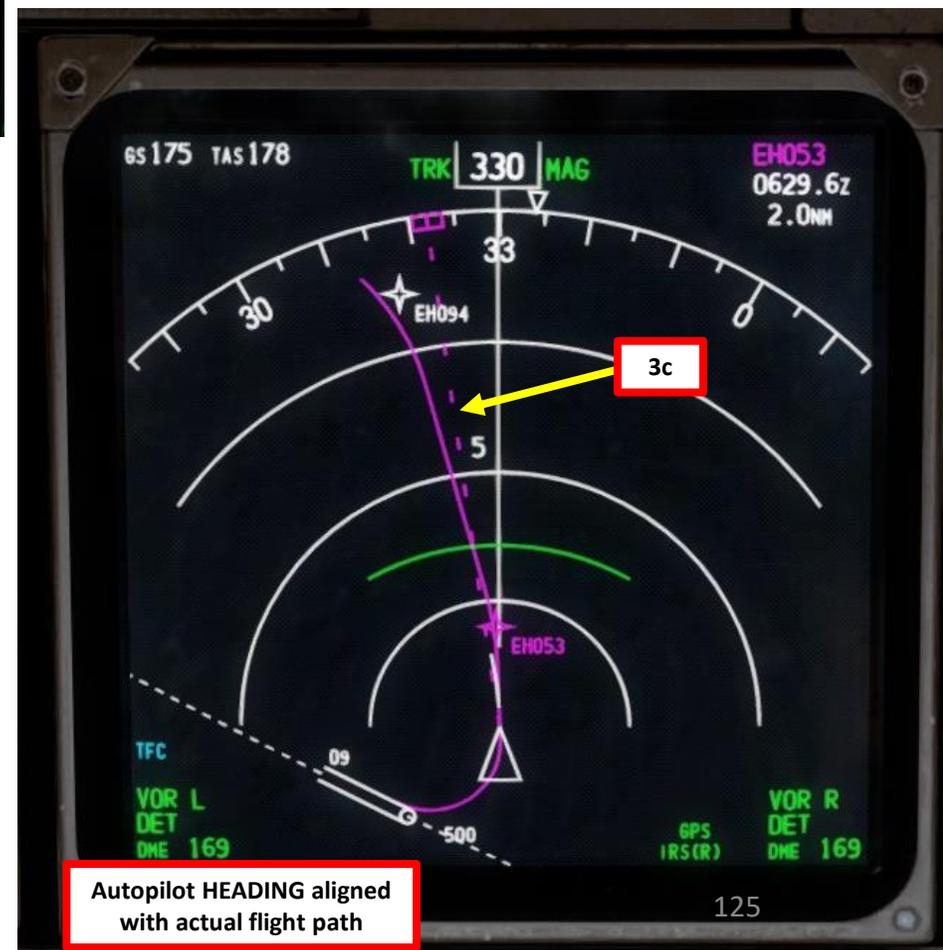
Autopilot HEADING aligned with actual flight path
