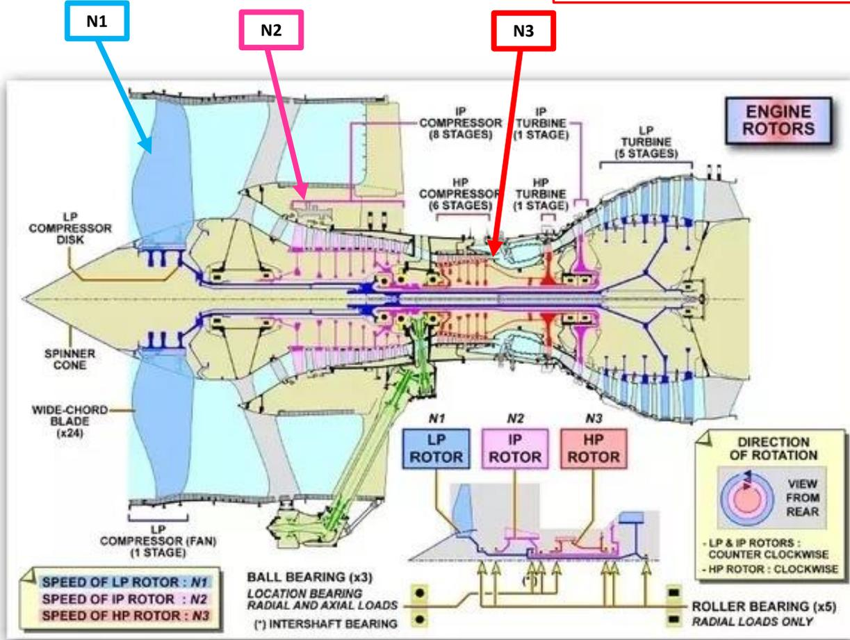
Intermediate-pressure compressor and intermediate-pressure turbine are driven by the same shaft. This is N2 speed in percentage of maximum RPM.
