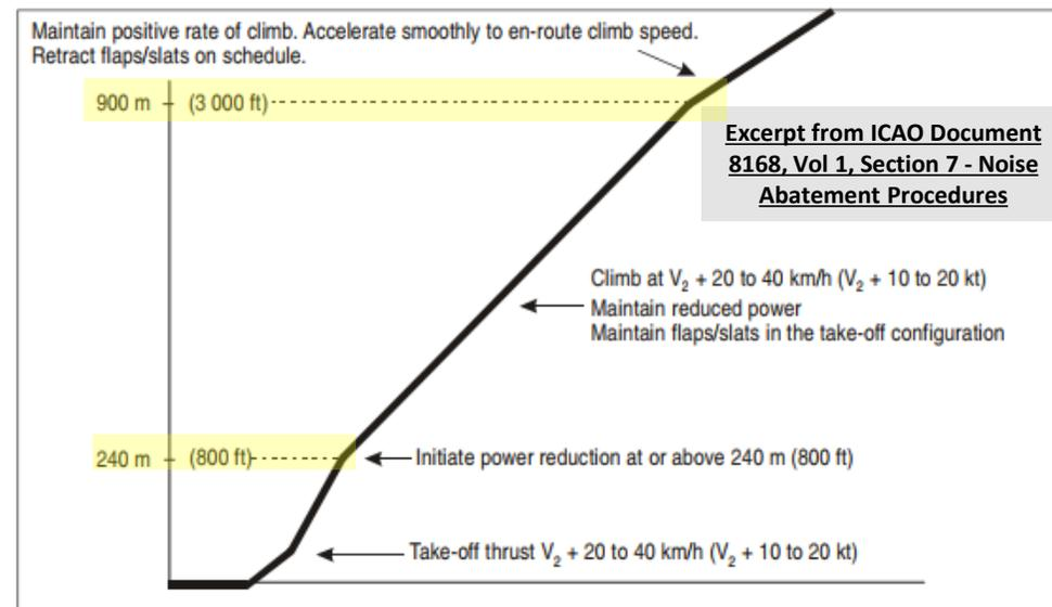
Figure I-7-3-App-1. Noise abatement take-off climb — Example of a procedure alleviating noise close to the aerodrome (NADP90)
