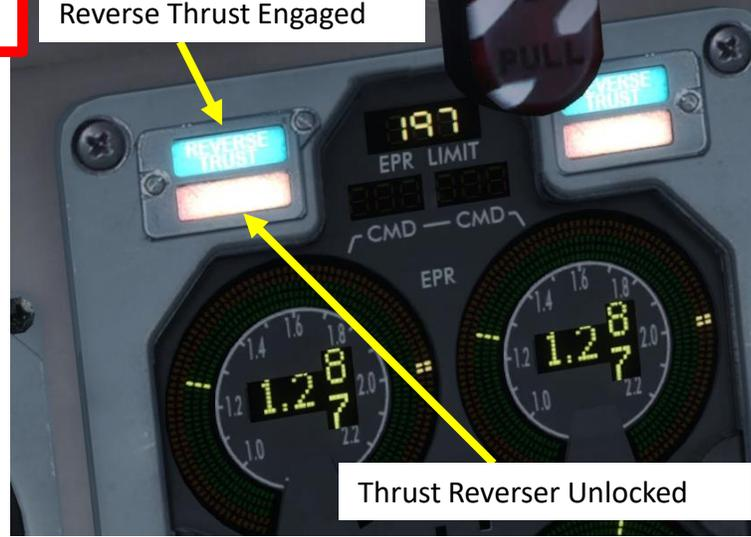
Thrust Reverser Unlocked
