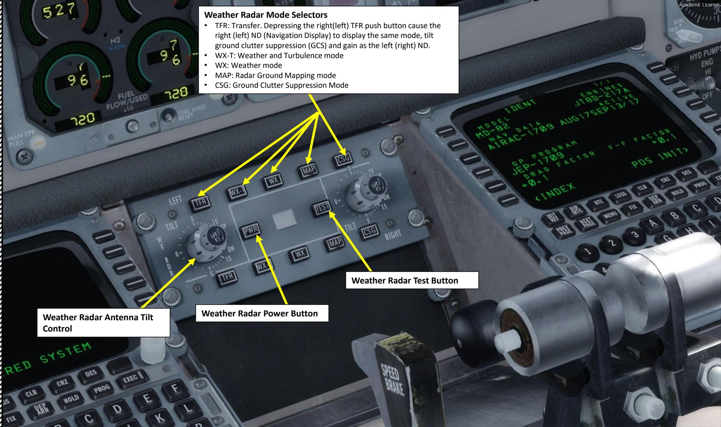
Weather Radar Antenna Tilt Control
