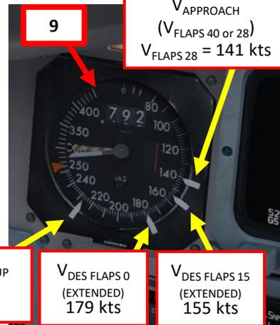
V<sub>DES</sub> FLAPS UP (RETRACTED) 228 kts
