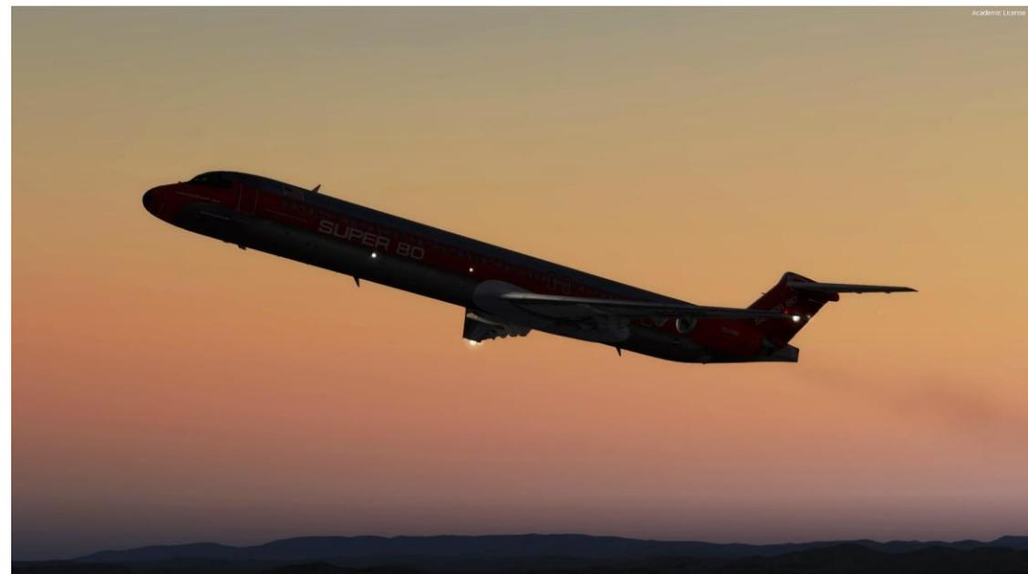
The Maddog is either loved or hated. The much maligned MD-80 (or DC-9 Super 80, to be exact) is a good aircraft, but is more difficult to fly since the control surfaces are not operated hydraulically, but are flown with cable actuated trim tabs. As a result, yoke inputs have a delayed reaction, and overcontrolling is likely. The rudder, however, is hydraulically powered. This makes flying an approach in unstable air is much more challenging in the MD than in a Boeing.
