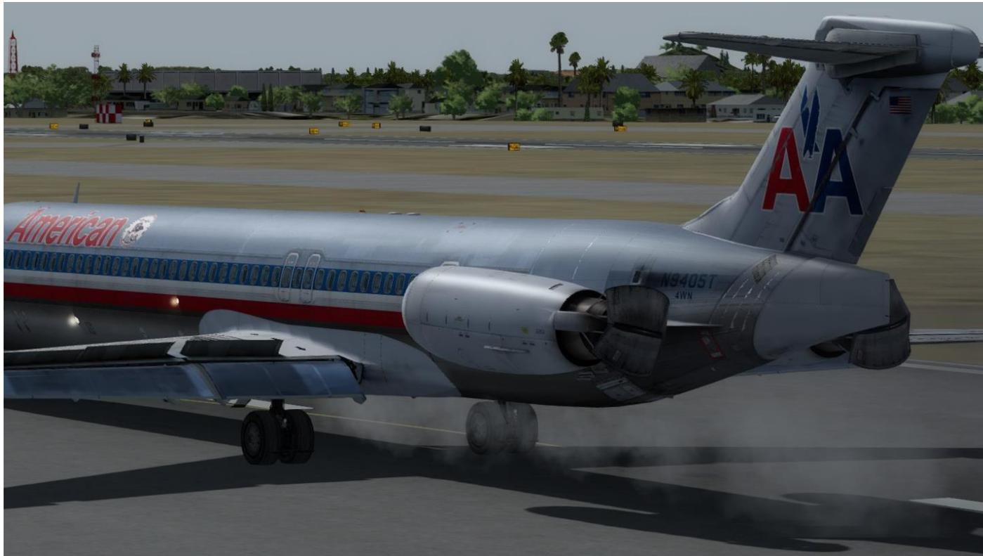
Thrust Reversers Armed & Deployed
