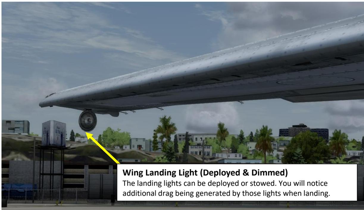
**Wing Landing Light (Deployed & Dimmed)**
