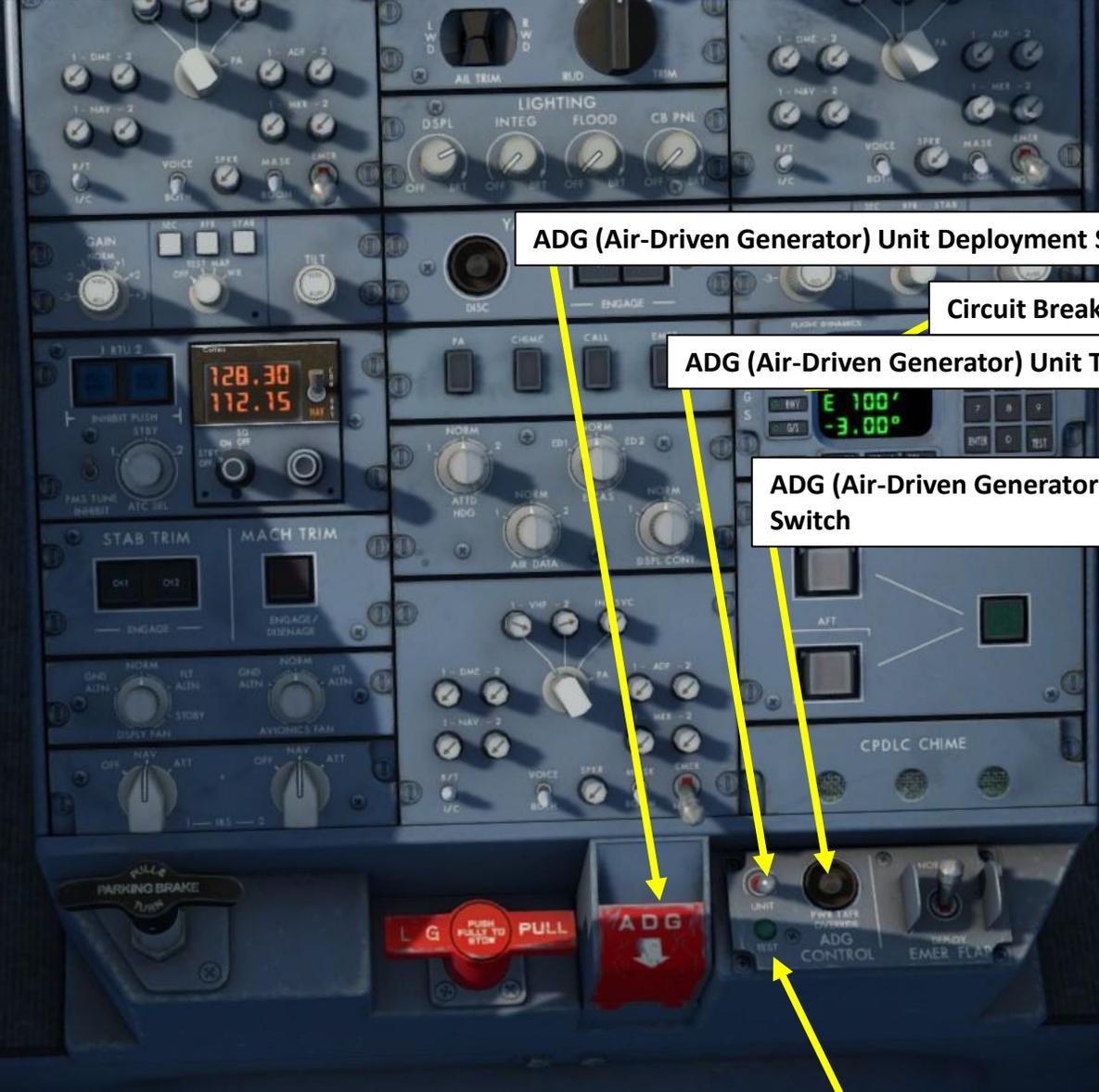
ADG (Air-Driven Generator) Unit Deployment Switch
