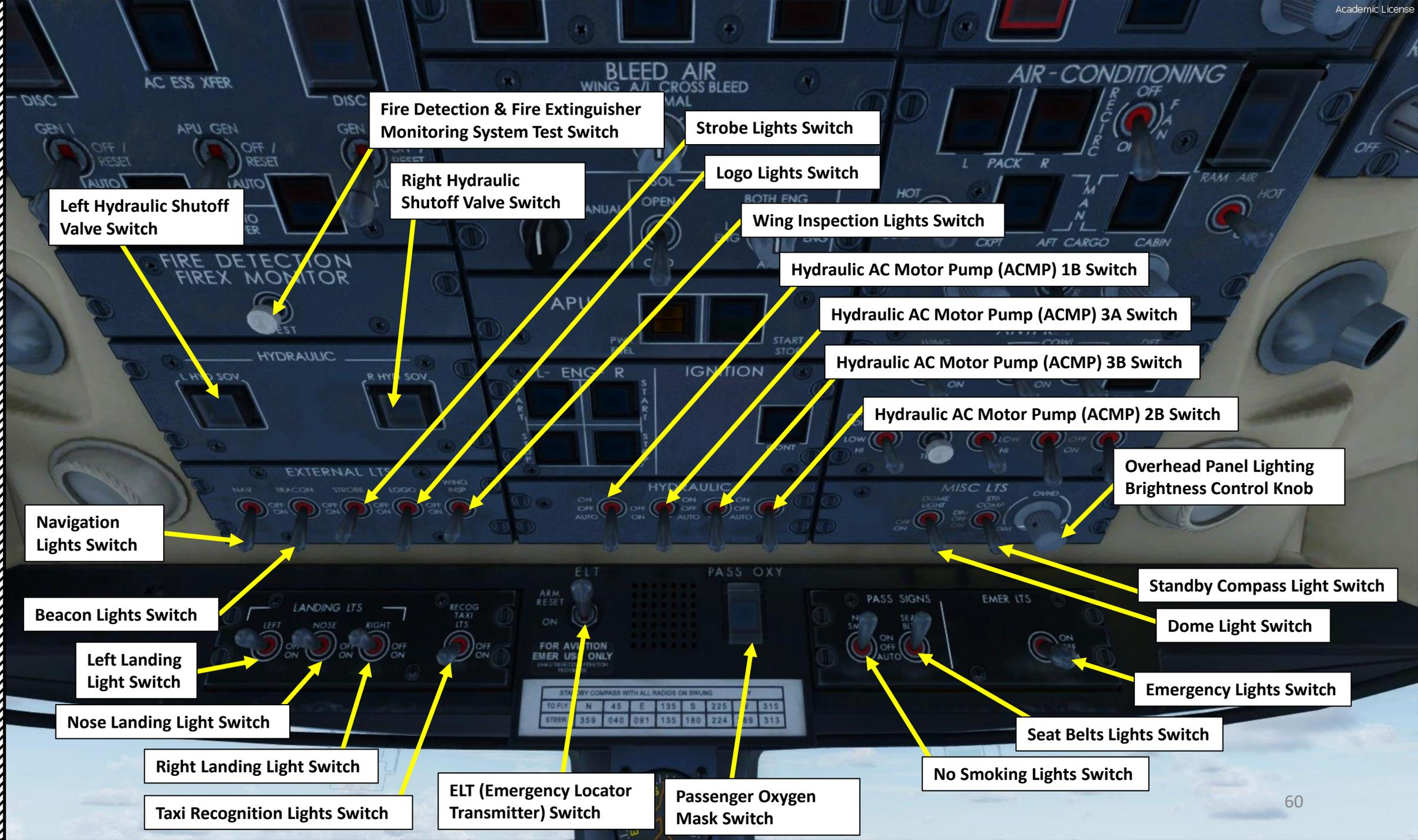
Left Hydraulic Shutoff Valve Switch
