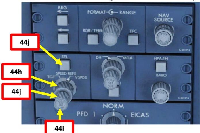
**V<sub>1</sub>** is the Decision Speed (minimum airspeed in the takeoff, following a failure of the critical engine at V<sub>EF</sub>, at which the pilot can continue the takeoff with only the remaining engines), **V<sub>R</sub>** is the rotation speed (airspeed at which the pilot initiates rotation to obtain the scheduled takeoff performance), and **V<sub>2</sub>** is Takeoff Safety Speed (minimum safe airspeed in the second segment of a climb following an engine failure at 35 ft AGL).
