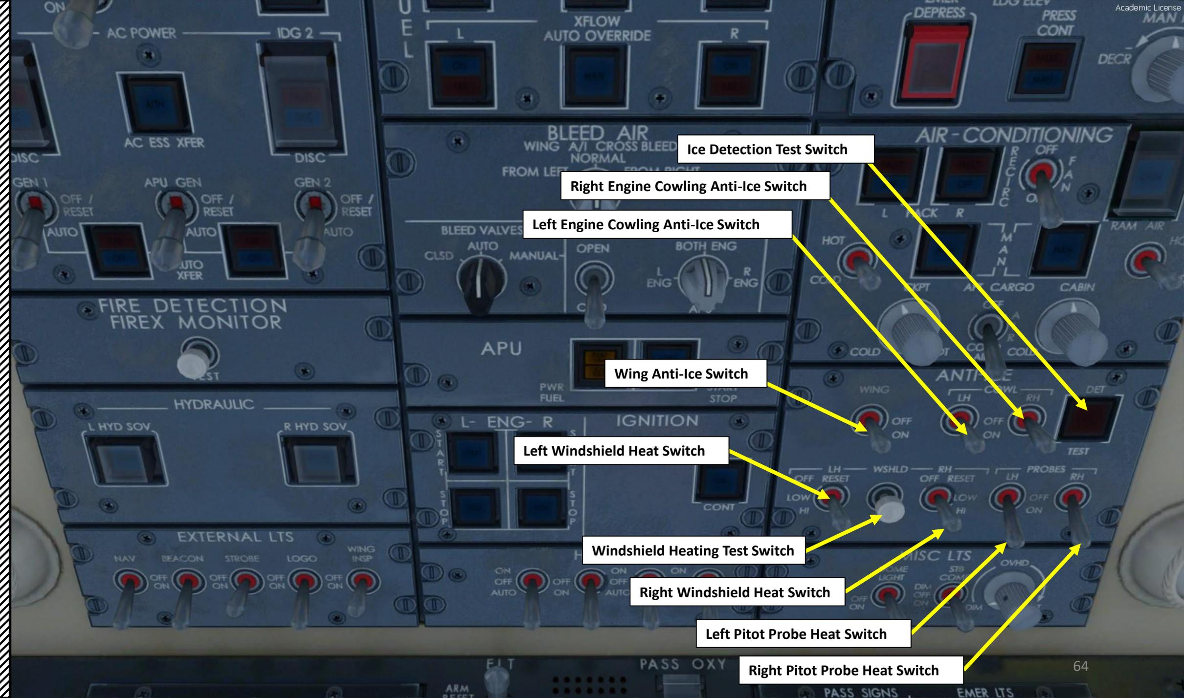
Ice Detection Test Switch
