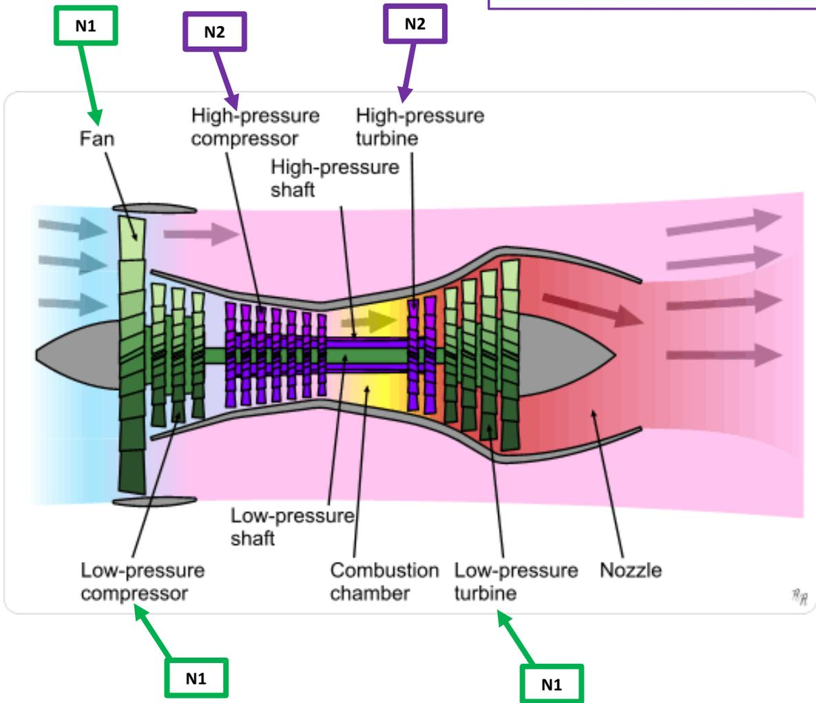
Fan, low-pressure compressor and low-pressure turbine are driven by the same shaft. This is N1 speed in percentage of maximum RPM.
