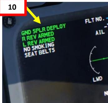
Thrust Reversers Armed & Deployed
