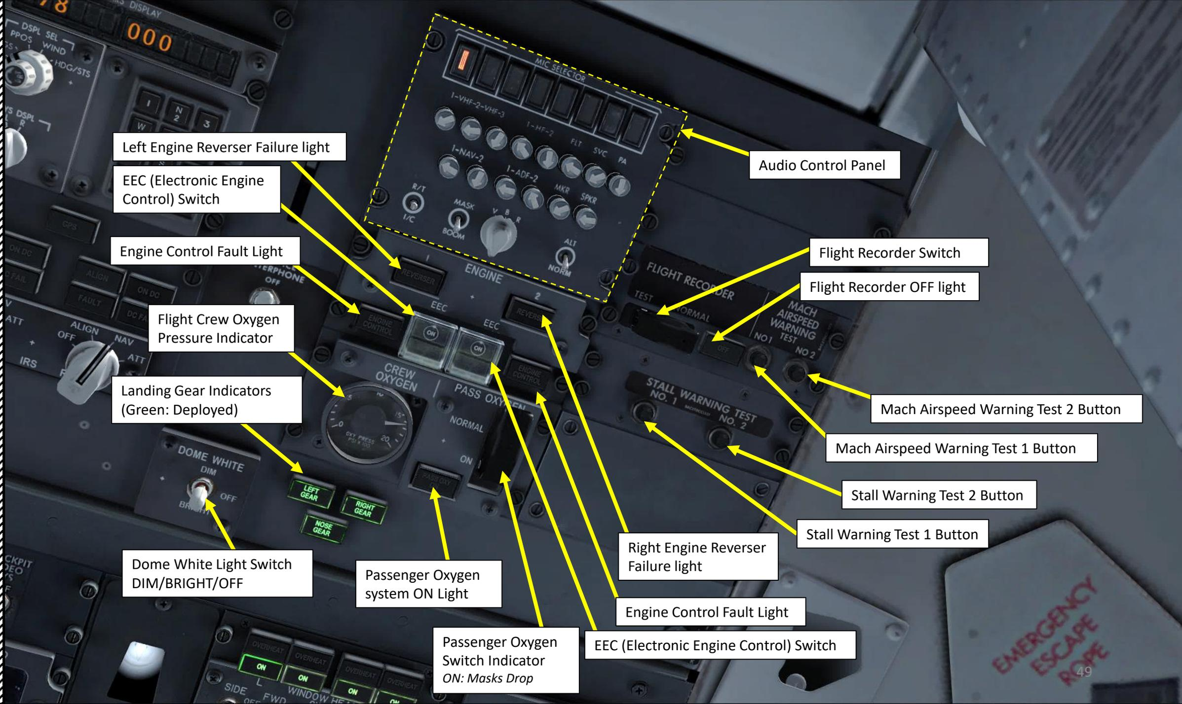
Left Engine Reverser Failure light
