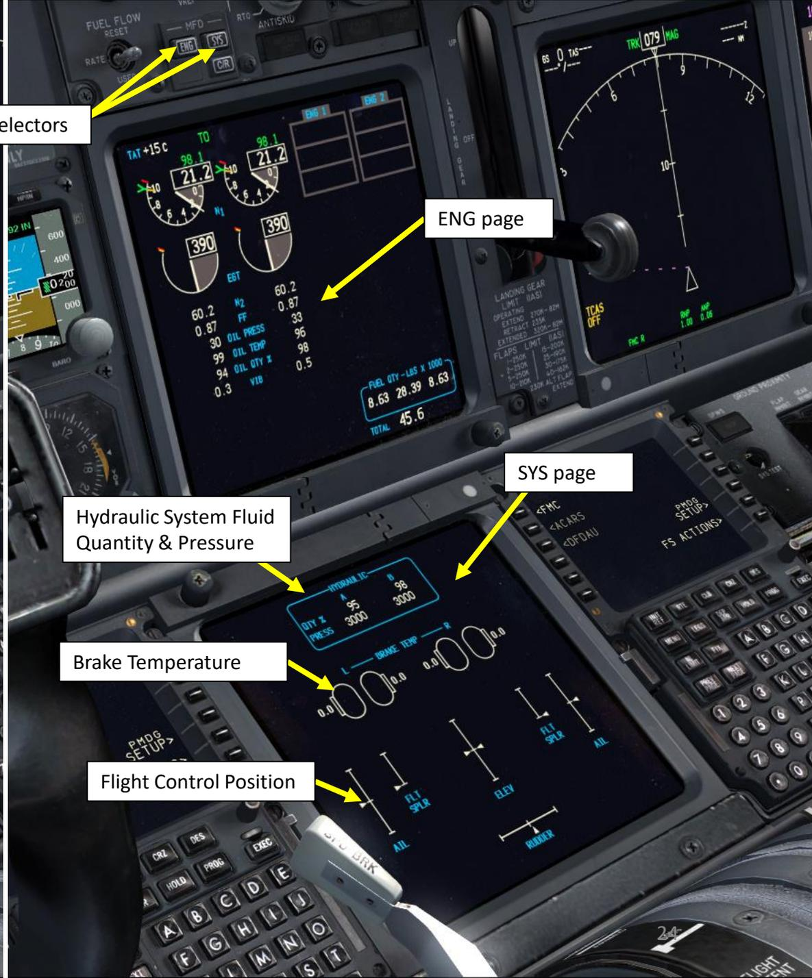
Hydraulic System Fluid Quantity & Pressure
