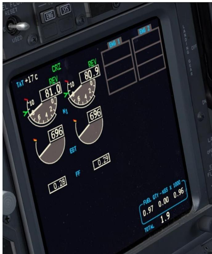
The Thrust Reverser lever can be moved by pressing and holding the “Throttle (decrease quickly)” control mapped to your joystick. Make sure that the “Repeat” slider is set fully to the right. The default key binding is “F2”.
