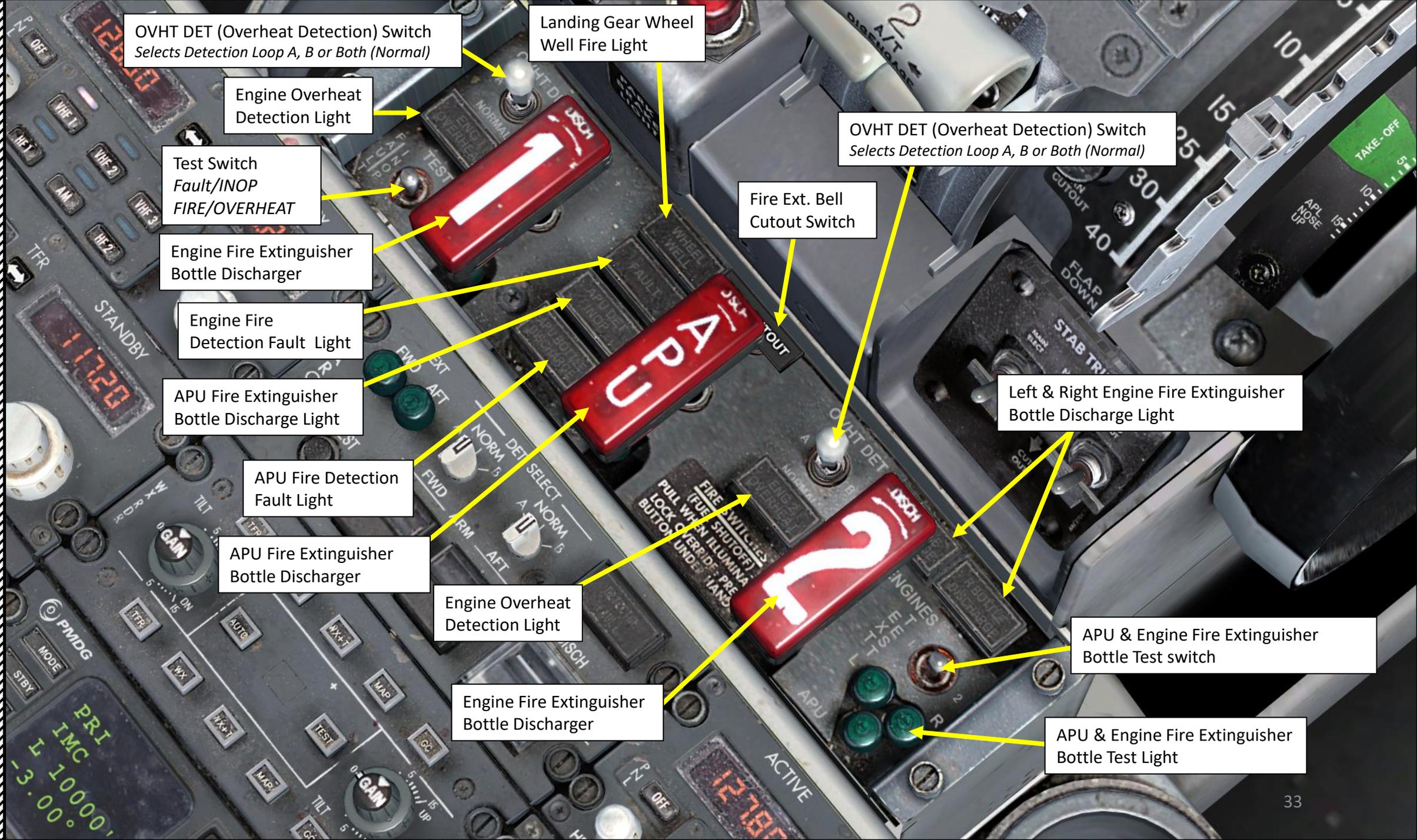
OVHT DET (Overheat Detection) Switch
