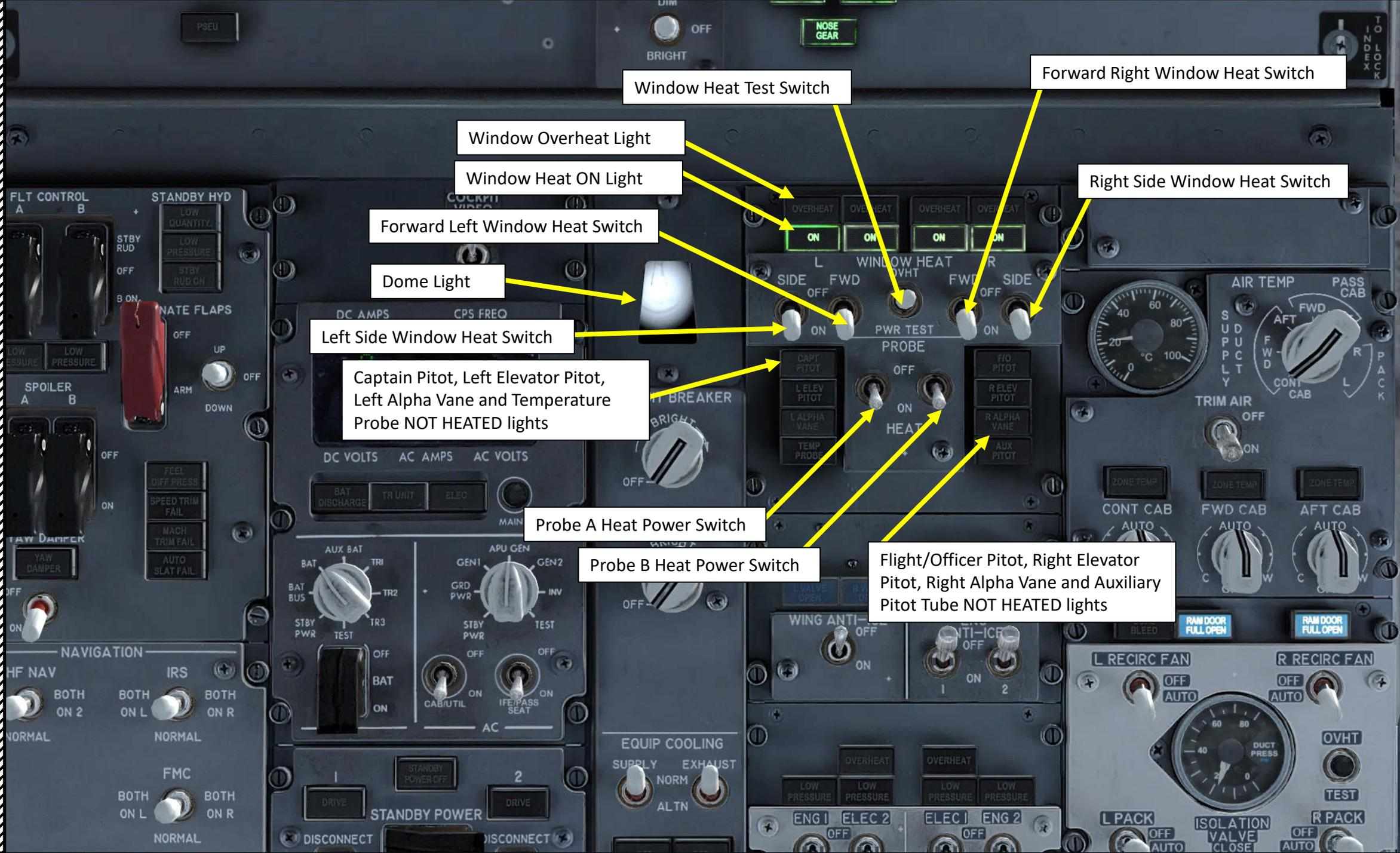
Window Heat Test Switch
