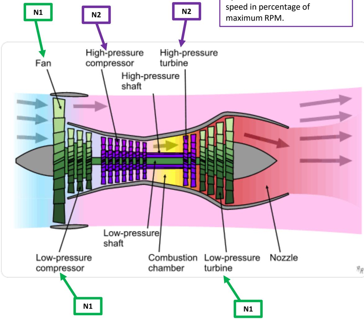
High-pressure compressor and high-pressure turbine are driven by the same shaft. This is N2 speed in percentage of maximum RPM.
