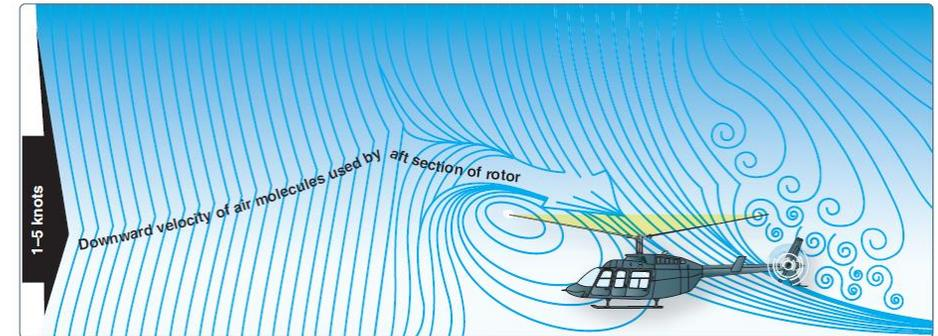
The airflow pattern for 1-5 knots of forward airspeed. Note how the downwind vortex is beginning to dissipate and induced flow down through the rear of the rotor system is more horizontal.
