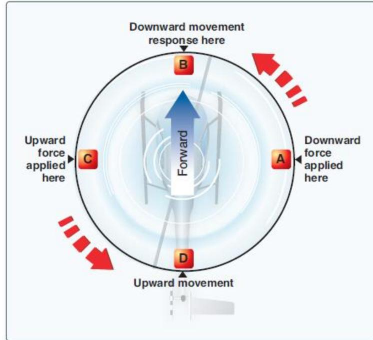
Figure 2-28. Gyroscopic precession.
