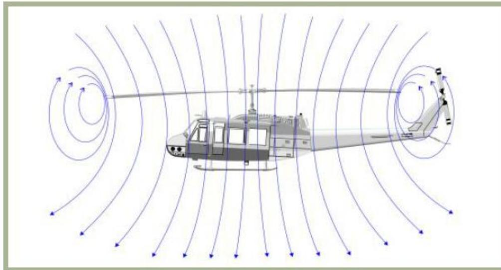
**Figure 3.13. Airflow When Out of Ground Effect**
