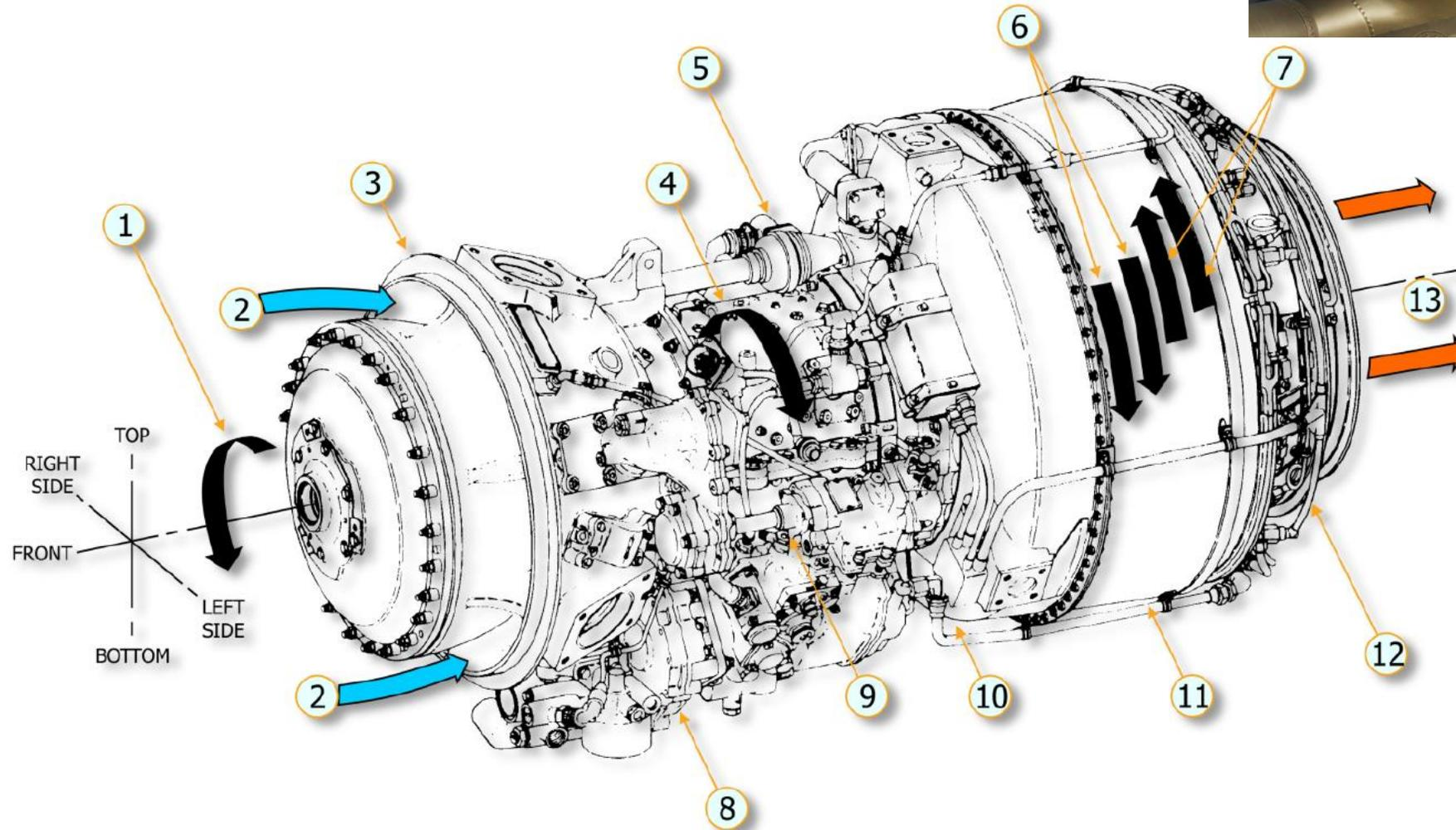
1. Rotation of Output Gearshaft
