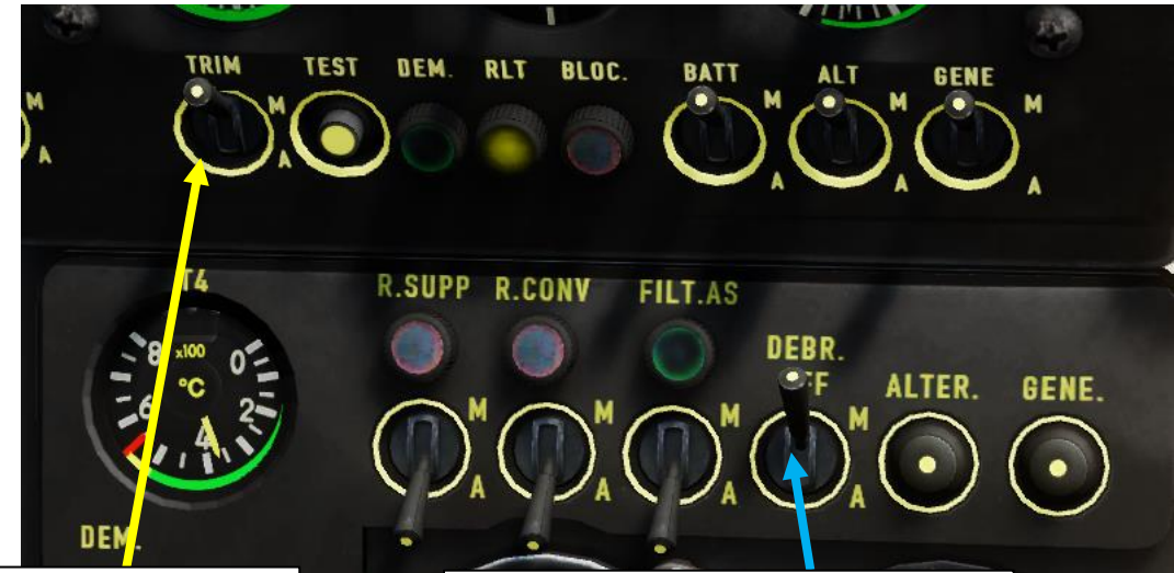
Trim Actuator Switch • M = Marche = ON (UP) • A = Arrêt = OFF (DOWN)
