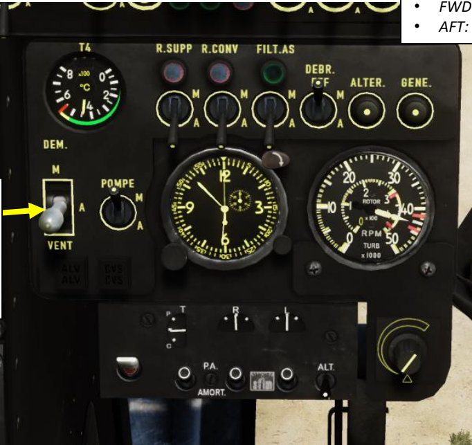
Starter/Ventilation (Démarrreur) Switch M = Marche = ON (UP) A = Arrêt = OFF (MIDDLE) VENT = Ventilation, Dry Crank (DOWN)
