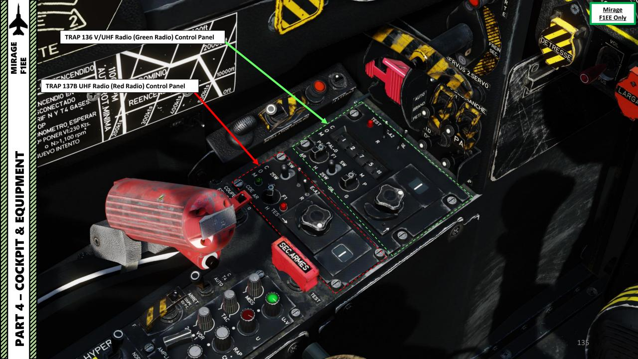
Main Fuel Cock / Fuel Shutoff Valve (Robinet Coupe-Feu) Switch
