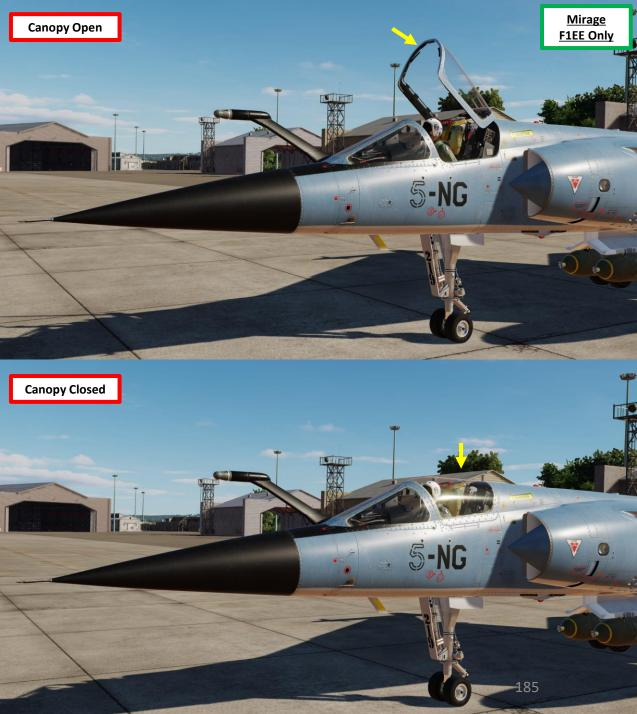
18. Once the canopy is lowered, push Canopy Lock lever FWD to lock and seal the cockpit. • Confirm P CAB (Cabin Pressurization) Warning Light is extinguished.
