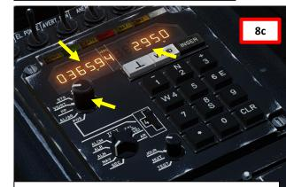
VS/RT: 365 kts Ground Speed, True Heading 295
