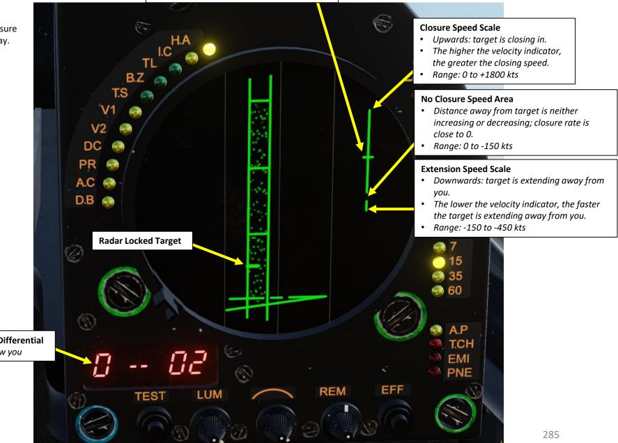
Radar Locked Target Elevation/Altitude Differential
