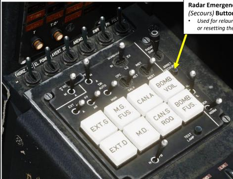
**Radar Emergency Transmission** (Secours) Button • Used for relaunching transmission
