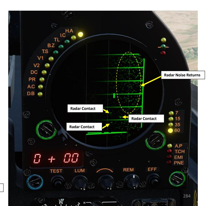
When the **radar has locked a target**, closure speed information is visible on the radar display.
