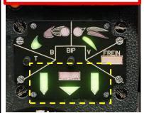
Landing Gear Control Lever (Palette de Commande de Train d'Atterrissage) • UP: Landing Gear Retracted
