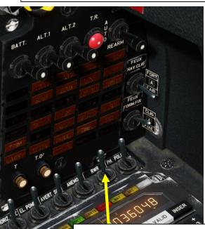
Radar Detector (Radar Warning Receiver) Switch
