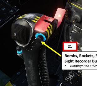
Bombs, Rockets, Missile & **Sight Recorder Button** Binding: RALT+SPACE
