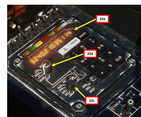
5 – UNI/INS (Unité de Navigation Inertielle / Inertial Navigation System) Alignment
