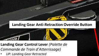
DOWN: Landing Gear Deployed
