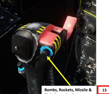
Bombs, Rockets, Missile & Sight Recorder Button • Binding: RALT+SPACE
