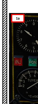
Afterburner (PC, Post-Combustion) INJ (Injection) Light Afterburner (PC, Post-Combustion) ON Light
