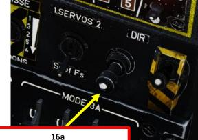
Nose Gear Weight On Wheels Pushed IN: High Gain/Sensitivity
