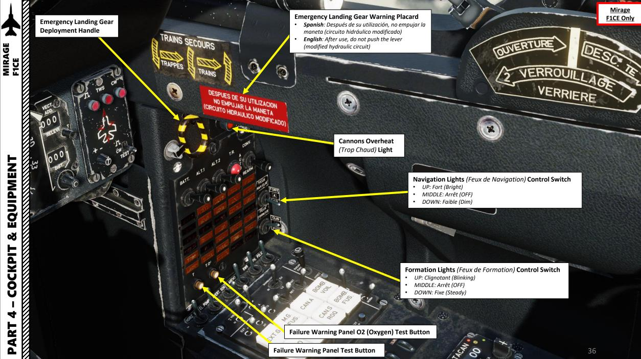
Failure Warning Panel Test Button
