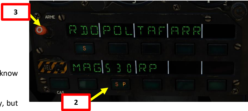
Missile Launched, Lost Lock PSIC Super 530 + Forced Illumination Mode
