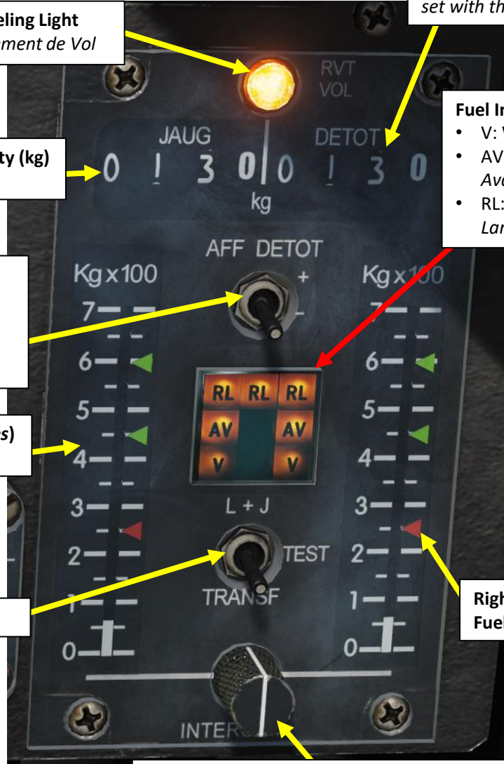
Internal Fuel Transfer Control (Not Functional) • Fuel cross-feed, used to keep fuel level balanced for different fuel tanks
