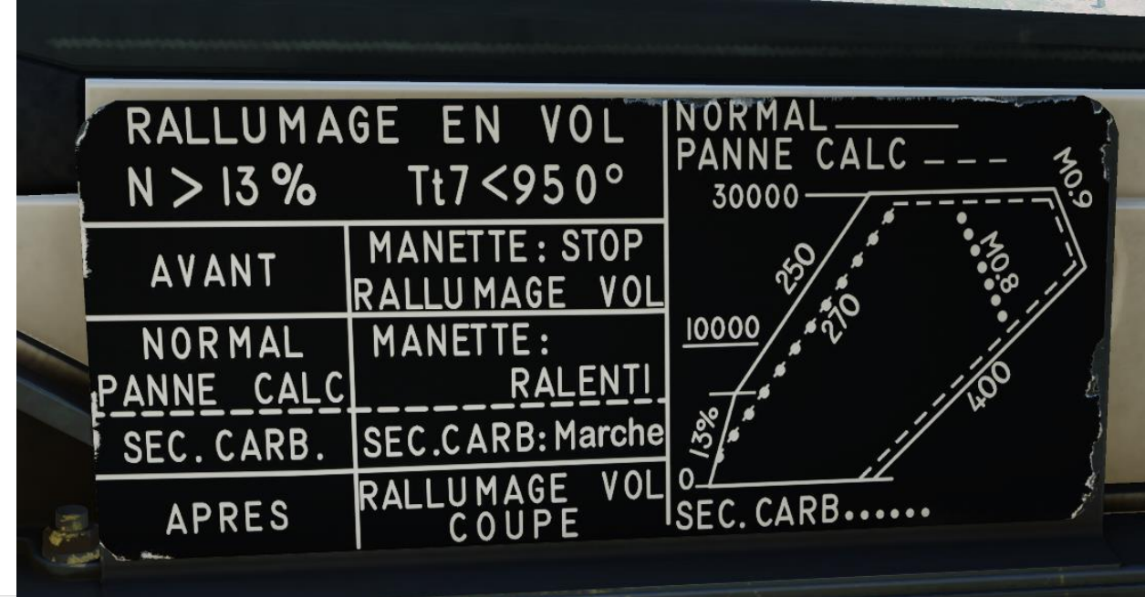
Allowable In-Flight Engine Relight Domain (Speed vs Altitude)
