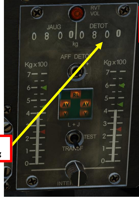
DETOT keeps decreasing despite fuel being taken from the tanker
