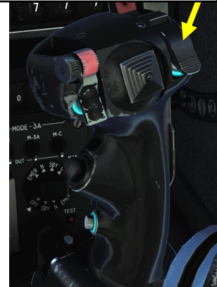
MAGIC Search / Vertical Fix Button (Nav Update / Magic Unlock) (can be used to switch Magic II Search Mode)
