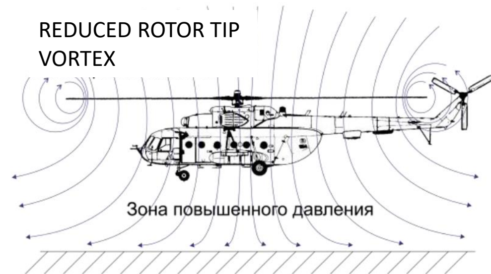
Fig. 9.17. Airflow when in ground effect
