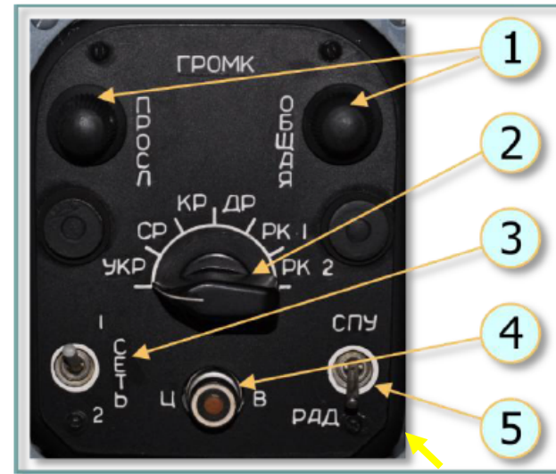
Рис. 9.89. SPU-7 control panel:
