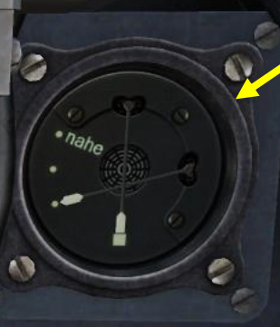
Supercharger Pressure Gauge (ATA) • Similar to Boost or Manifold Pressure
