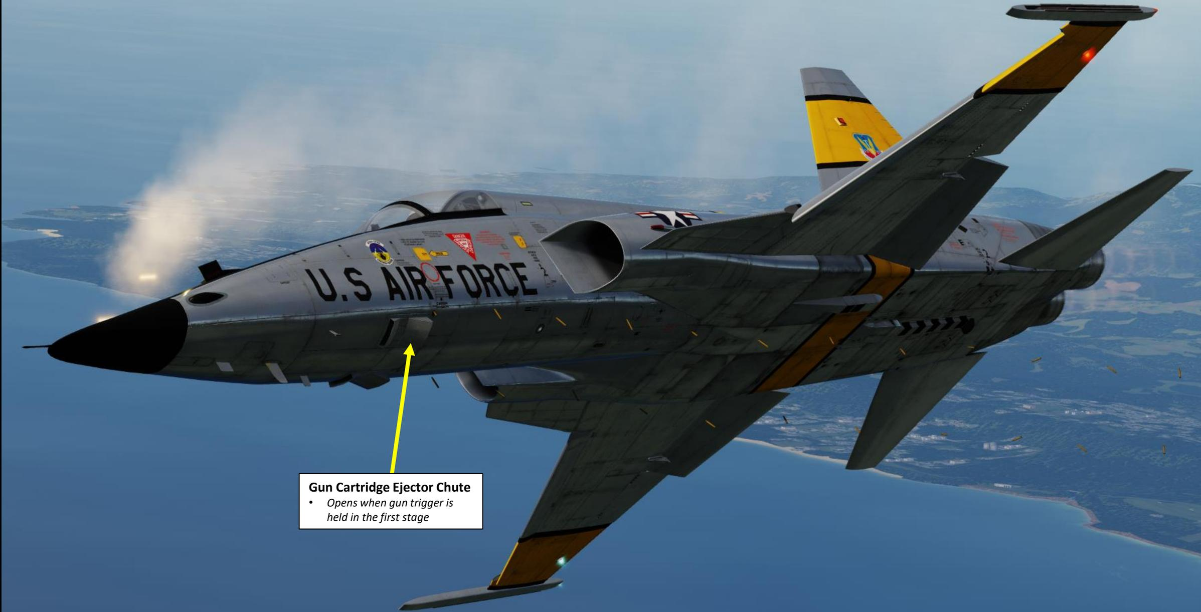
**Gun Cartridge Ejector Chute**
