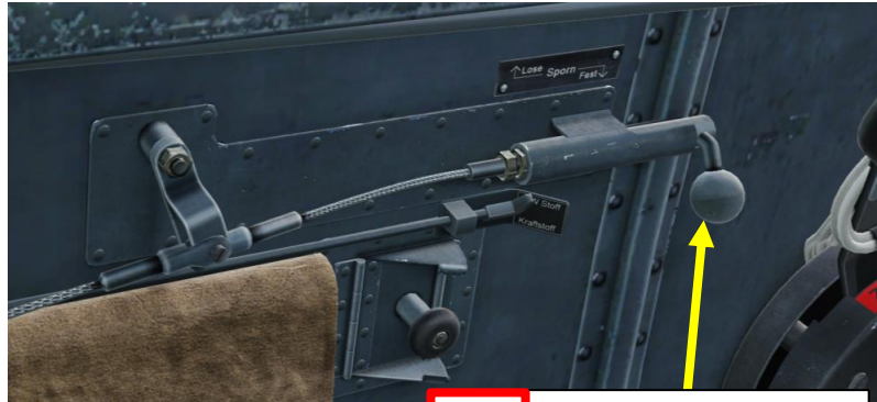
2 Tailwheel Locked ("L-shaped" position)
