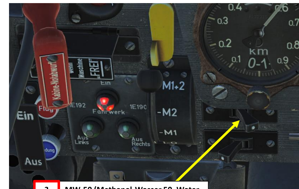
MW-50 (Methanol-Wasser 50, Water-Methanol Injection) Switch
