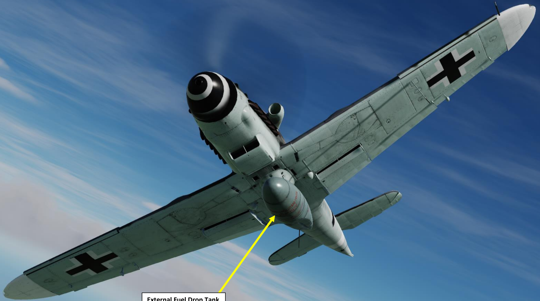
External Fuel Drop Tank (300 L)
