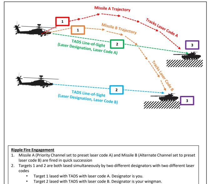
3. Missile A tracks laser code A until impact / Missile B tracks laser code B until impact
