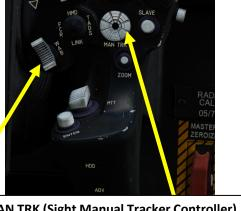
MAN TRK (Sight Manual Tracker Controller) Switch, also known as "Thumb Force Controller"
