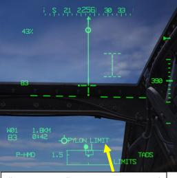
"PYLON LIMIT" Message is visible if pylon limits are exceeded
