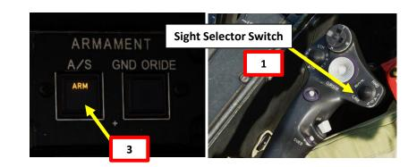
MAN TRK (Sight Manual Tracker Controller) Switch, also known as "Thumb Force Controller"
