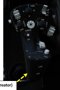
LMC (Linear Motion Compensator) **Button (Opposite Side)**
