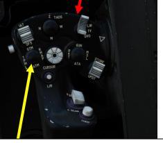
FCR (Fire Control Radar) Mode Selector FWD: GTM (Ground Targeting Mode) • AFT: **ATM** (Air Targeting Mode)
