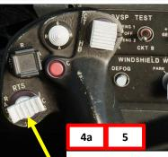
Floor-Mounted Radio Transmit Switch
