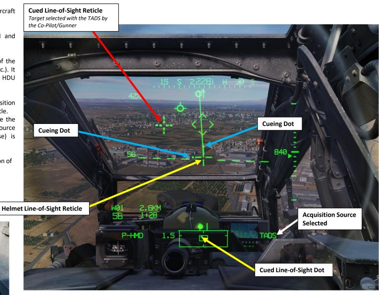
The HDU (Helmet Display Unit) can overlay calibrated video data from Forward-Looking Infrared (FLIR) or Day Television (DTV) sensors. The video data can come from the TADS (Target Acquisition & Designation Sight) or the PNVS (Pilot Night Vision System) depending on what video source is selected. Keep in mind that the PNVS and the TADS are two independent sensors.
