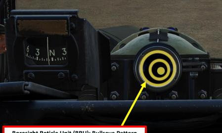
Boresight Reticle Unit (BRU): Bullseye Pattern Used to align/boresight HDU (Helmet Display Unit)
