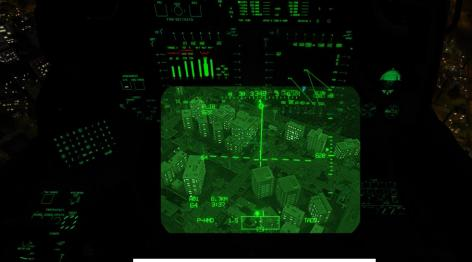
The PNVS allows you to see through the cockpit due to the position of the FLIR sensor.
