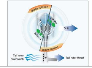
A tail rotor is designed to produce thrust in a direction opposite torque. The thrust produced by the tail rotor is sufficient to move the helicopter laterally.
