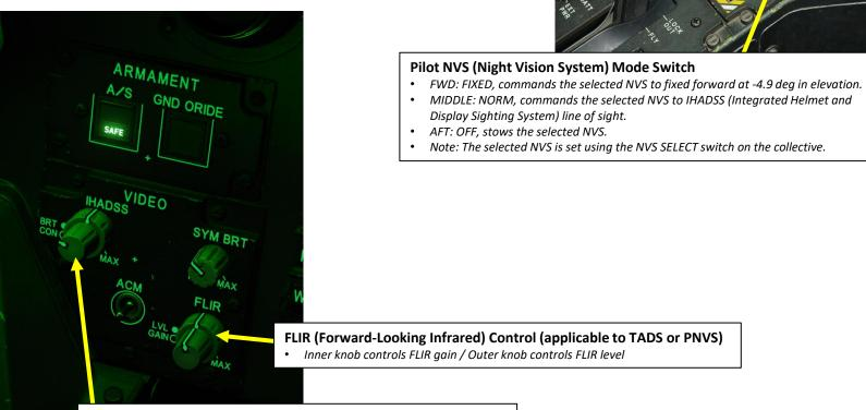
IHADSS (Integrated Helmet and Display Sighting System) Knobs • Inner knob controls video contrast / Outer knob controls video brightness.
