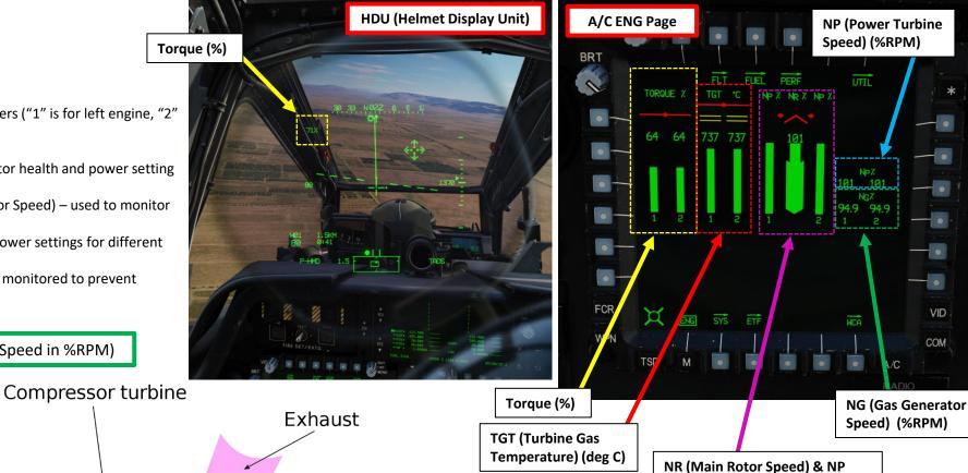
**NG** (Gas Generator / Compressor Rotation Speed in %RPM)
