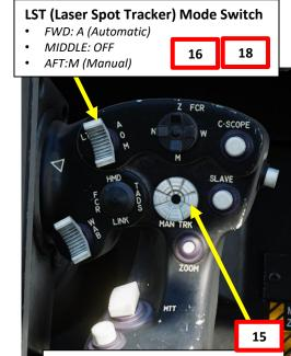
MAN TRK (Sight Manual Tracker Controller) Switch, also known as "Thumb Force Controller"
