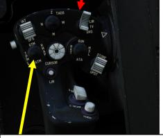
FCR (Fire Control Radar) Mode Selector FWD: GTM (Ground Targeting Mode)
