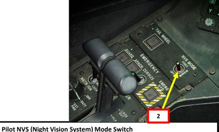
• FWD: FIXED, commands the selected NVS to fixed forward at -4.9 deg in elevation. MIDDLE: NORM, commands the selected NVS to IHADSS (Integrated Helmet and Display Sighting System) line of sight. AFT: OFF, stows the selected NVS. Note: The selected NVS is set using the NVS SELECT switch on the collective. **PNVS (Pilot Night** Vision System) Overlay 195
