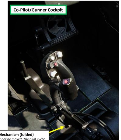
Stick (Cyclic) Folding Mechanism (folded) When folded, cyclic cannot be moved. The pilot cyclic should override the co-pilot/gunner's cyclic input.
