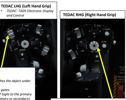
MAN TRK (Sight Manual Tracker Controller) Switch, also known as "Thumb Force Controller"
