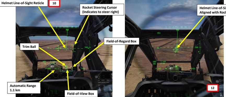
Helmet Line-of-Sight Reticle Aligned with Rocket Steering Cursor
