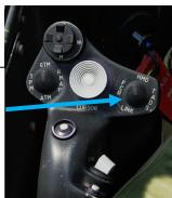
For the co-pilot/gunner, the TDU (TEDAC Display Unit) Symbology Brightness Adjustment Rocker Switch is used to adjust the HDU brightness.
