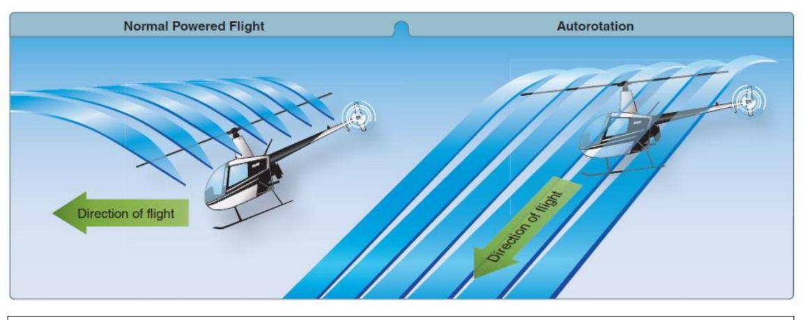
During an autorotation, the upward flow of relative wind permits the main rotor blades to rotate at their normal speed. In effect, the blades are "gliding" in their rotational plane.
