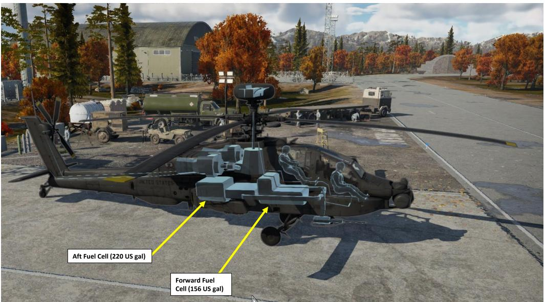
A 230-gallon external fuel tank can be mounted on each of the four stub wing pylons. The external fuel tank mounted under the left inboard pylon feeds the forward fuel cell, and external fuel tank mounted under the right inboard pylon feeds the aft fuel cell. If an additional two fuel tanks are mounted under the outboard pylons, the outboard external fuel tanks feed fuel to the inboard-mounted external fuel tanks.
