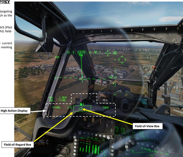
The **Helmet Line-of-Sight Reticle** provides a fixed reference for aircraft pitch attitude and for weapon aiming. The reticle flashes when:
