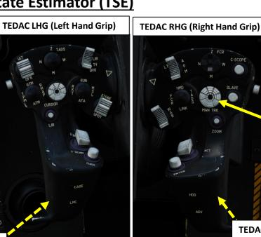
MAN TRK (Sight Manual Tracker Controller) Switch, also known as "Thumb Force Controller"
