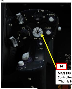
26 TE MAN TRK (Sight Manual Tracker Controller) Switch, also known as "Thumb Force Controller"
