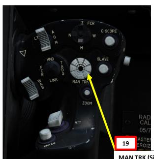
MAN TRK (Sight Manual Tracker Controller) Switch, also known as "Thumb Force Controller"
