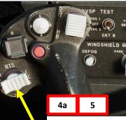
Floor-Mounted Radio Transmit Switch
