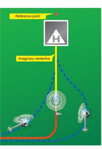
Figure 9-20. Plan the turn to final so the helicopter rolls out on an imaginary extension of the centerline for the final approach path. This path should neither angle to the landing area, as shown by the helicopter on the left, nor require an S-turn, as shown by the helicopter on the right.
