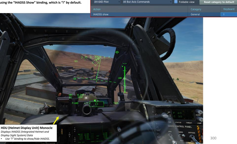
IHADSS (Integrated Helmet and Display Sighting System) SSU **Head-Tracking Sensors**
