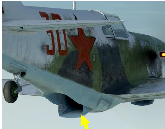
WATER RADIATOR OPEN
