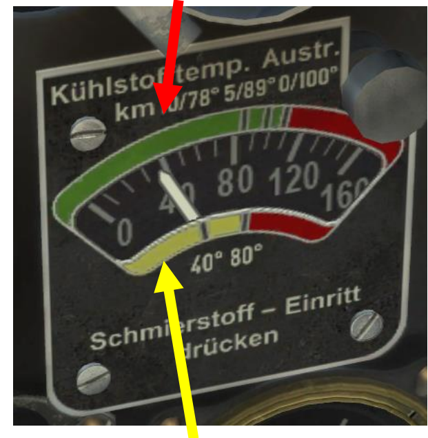
OIL INTAKE TEMPERATURE (DEG C)
